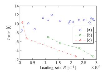
FIG. 4. MOT loading rate R plotted against  $1/\tau_{\rm ODT}$ , where  $\tau_{\rm ODT}$  is the lifetime in the dipole trap, for experimental situations (a): LIAD on for MOT loading, off for dipole trapping; (b): LIAD on for both; (c): no LIAD, dispensers on for both. Case (a) corresponds to a dipole trap lifetime independent of the MOT loading rate, whereas they are inversely related in cases (b) and (c).
