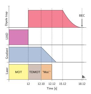
FIG. 2. (a): Sketch of the UHV chamber, showing the location of one of the pairs of LEDs with respect to the MOT and the reentrant viewports (VP), as well as the path of one of the ODT arms. (b): Time sequence of the experiment. We show from the top down the power of the ODT, the current in the LEDs, the magnetic gradient of MOT coils and the different cooling phases. TDMOT stands for Temporal Dark MOT and "Mol." for "optical molasses" (see Sec.II C).
