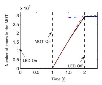
FIG. 5. Evolution of the loading of the MOT after extinction of the LEDs: the MOT is loaded for 1 s then the LEDs are turned off. The loading rate shown as a red (blue) dashed line is  $3 \times 10^6 \text{ s}^{-1} (8 \times 10^4 \text{ s}^{-1})$  when the LEDs are on (off).
