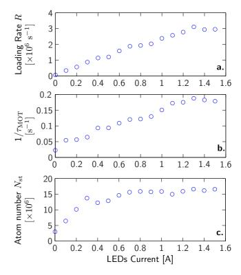
FIG. 3. (a): Loading rate R of the MOT; (b): Inverse of the loading time constant  $1/\tau_{\text{MOT}}$ ; (c): Steady–state atom number  $N_{\text{st}}$  for various LED currents. Statistical error bars are smaller than the dots and not shown.
