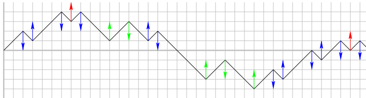
Fig. 3. Flips can increase the number of mismatches (red arrows), let it unchanged (blue arrows) or decrease it (green arrows). The two last are respectively called reversible and irreversible flips: they are the only ones performed during the cooling process.
