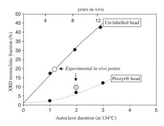
Fig. 6. Kinetics measured on polished 'non-aged' (see text) sections of the two heads at 134  $^{\circ}$ C, calculated at 37  $^{\circ}$ C from apparent activation energy, and compared with experimental in vivo points.
