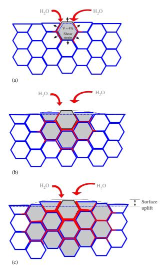
Fig. 2. Scheme of the ageing process occurring in a cross section, showing the transformation neighbor to neighbor. (a) Nucleation on a particular grain at the surface, leading to microcracking and stresses to the neighbors. (b) Growth of the transformed zone, leading to extensive microcracking and surface roughening. Transformed grains are gray. Red path represents the penetration of water due to microcracking around the transformed grains.
