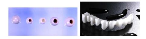
Fig. 1. Range of femoral heads dimensions allowed with zirconia (courtesy HTI, Decines, France) and example of a zirconia dental bridge (courtesy Diatomic, Louey, France).
