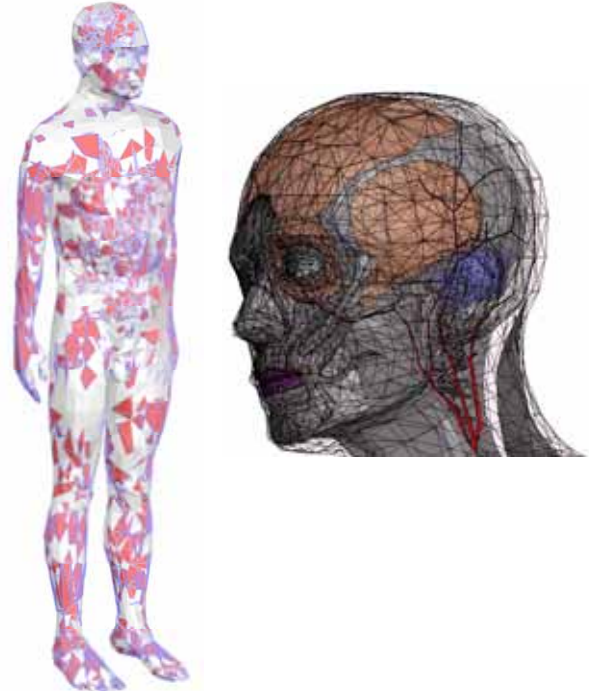
Fig. 3. Left: the computational phantom; the elements eliminated for post-processing are rendered in red. Right: details of the 2mm resolution phantom.
