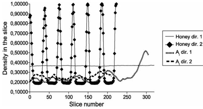
Fig. 3. Examples of volume fraction profiles of the ceramic as a function of the slice number in two samples (*Honey* and *A<sub>1</sub>* samples) and in two directions for each material.
