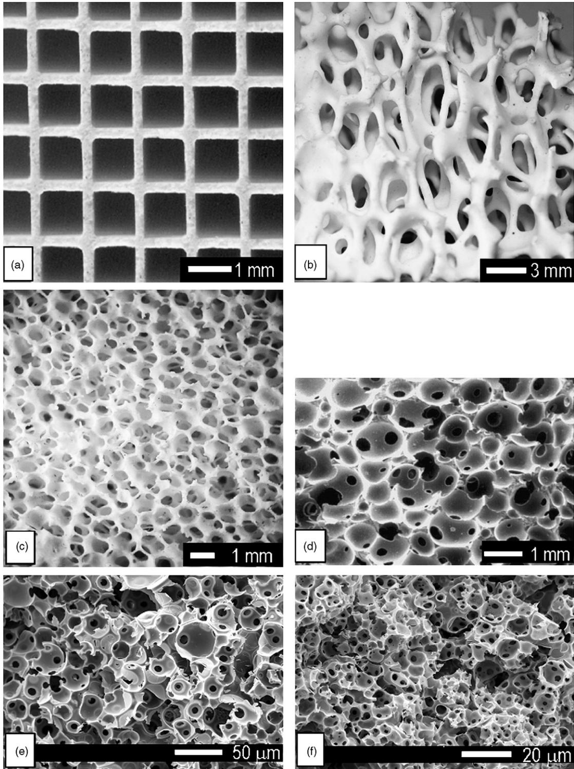
Fig. 1. General morphology of the samples used. Optical microscopy images of samples: (a) *Honey*; (b) *A<sub>1</sub>*; (c) *A<sub>m</sub>*. SEM micrographs of samples: (d) *S<sub>m</sub>*; (e) *S<sub>50</sub>*; (f) *S<sub>10</sub>*.
