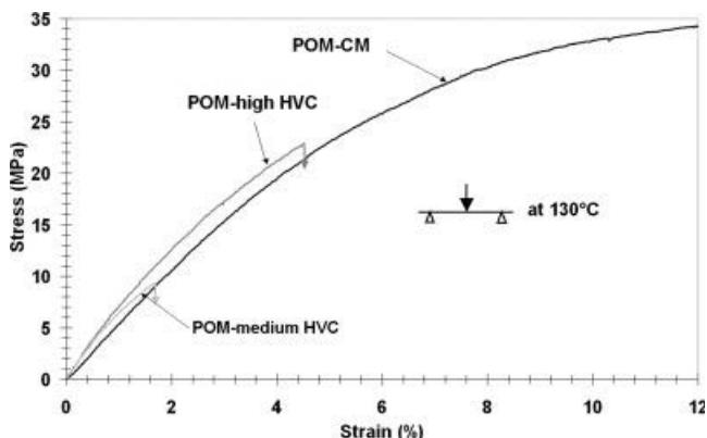
**Figure 16** Stress-strain curves from three-point-bending tests at 130°C.
