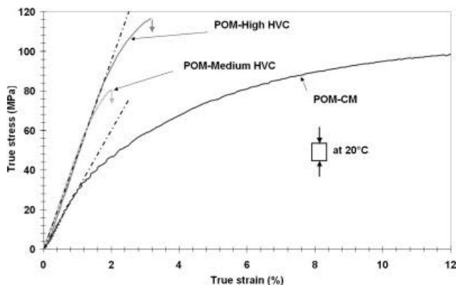
**Figure 14** Stress–strain curves from compressive tests at 20°C.
