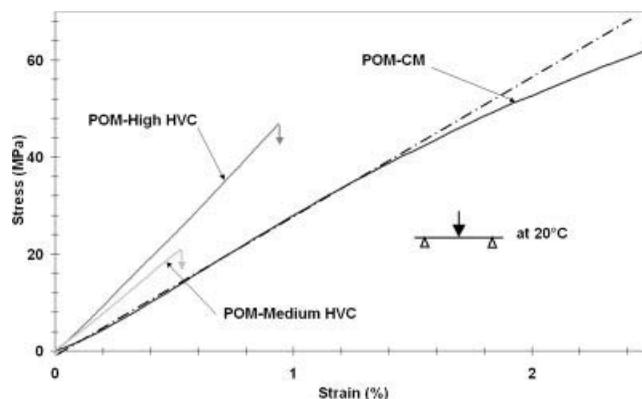
**Figure 6** Stress–strain curves from three-point-bending tests at  $20^\circ\text{C}$ .
