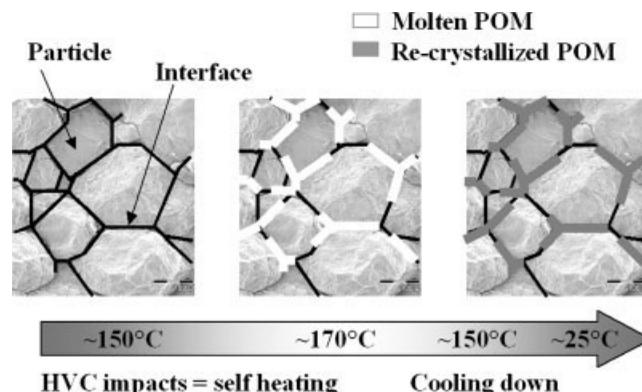
**Figure 17** Schematic representation of the sintering mechanism.
