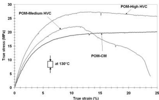
**Figure 15** Stress-strain curves from compressive tests at 130°C.
