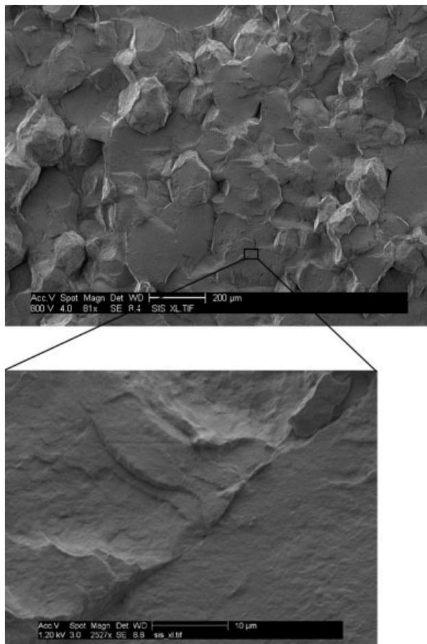
**Figure 11** LVSEM room-temperature fracture surface observation: POM-high HVC.
