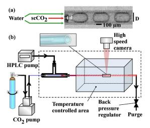
FIG. 1. (Color online) Coflowing setup developed for this study. (a) Typical observation of the flow with the insertion of a small diameter fused silica tubing in a larger one. *D* and *d* are the inner diameters of the large and the small tubing, respectively. (b) General setup including two high pressure pumps, a T connector for the insertion of the small silica tubing in the larger one, a temperature-controlled area and a back pressure regulator.
