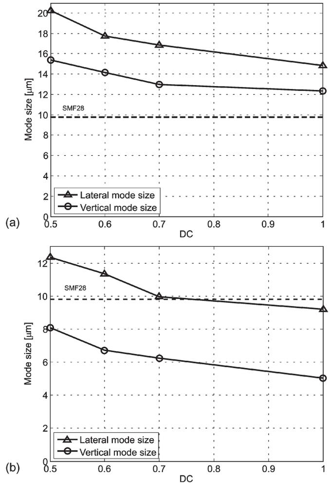
Fig. 3. Measurement of the lateral and vertical mode sizes (at  $1/e$  of the field maximum) of SWGs as a function of DC with  $W = 5 \mu\text{m}$  and  $P = 15 \mu\text{m}$  for two samples fabricated with (a) 3.5% and (b) 2.8% of LB. The dotted line refers to the mode size of the output fiber SMF28.
