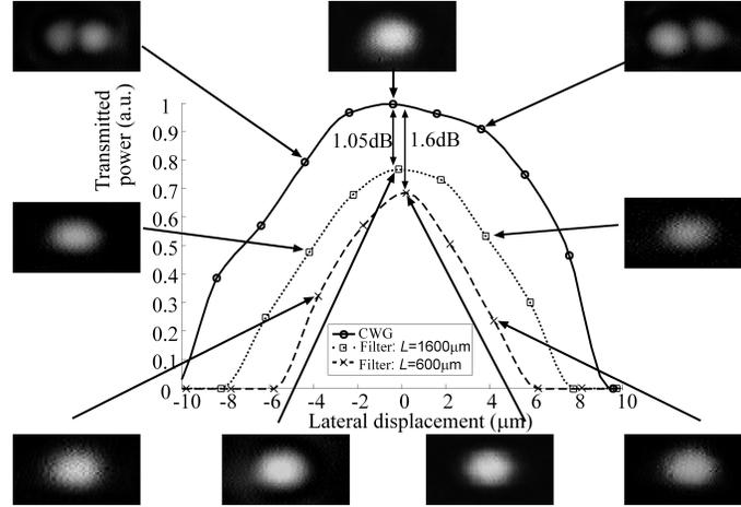
Fig. 5. Transmitted power measured as a function of the lateral displacement of the input objective for a continuous and two filtered WGs with taper length  $L_A = 0.6$  mm (dashed line) and  $L_B = 1.6$  mm (dotted line). Camera images confirm the single-mode behavior of the filtered waveguides. Symbols represent measured values; lines are for visual aid only.
