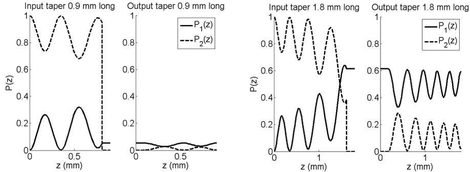
Fig. 3. Power evolution of the fundamental ( $P_1$ , solid line) and higher order ( $P_2$ , dashed lines) in the input and output tapers with  $L = 0.9$  mm (left) and 1.8 mm (right) when only the higher order mode is initially present.
