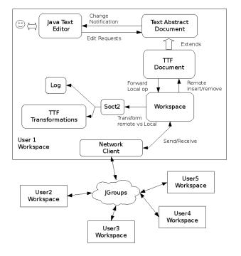
Figure 5. Graveyard architecture
