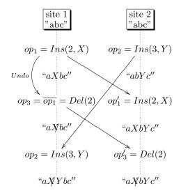
Figure 7. Using TTF functions with COT.
