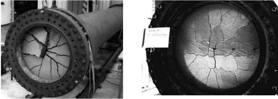
Figure 1.4. Shock tube failure trials for a plain or reinforced concrete slab (from [TOU 95a])
