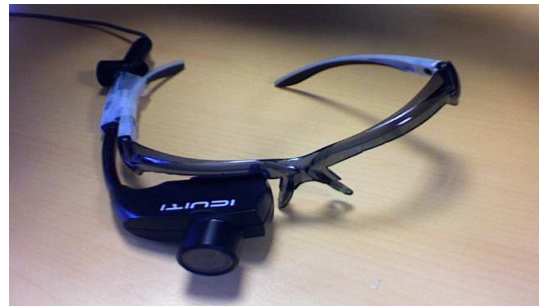
Fig. 4 Prototype of the Monocular Orthoscopic Video See-Through visualization system.
