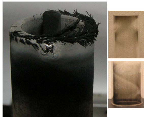
Figure 11. Photographs of the suit deposited on the injector (left) and on the walls of the quartz tube (right).
