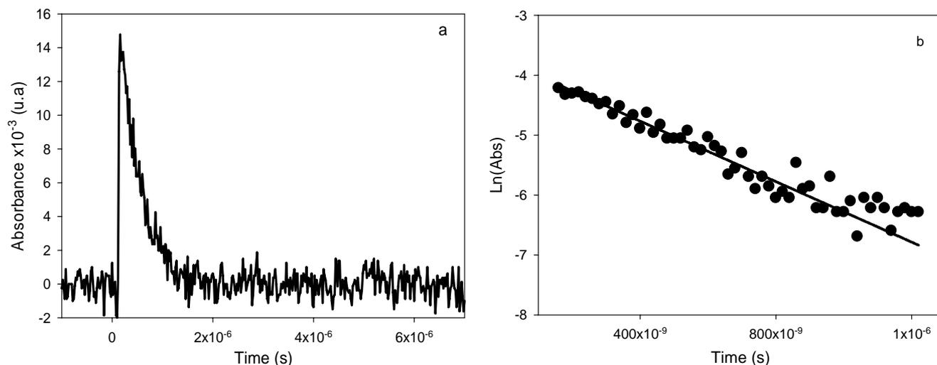
**Fig. 1.** (a) Transient absorption decay of the benzophenone triplet state ( $\lambda_{\text{obs}}=525$  nm) in deoxygenated aqueous solutions containing 4 mM of bromine. (b) Typical pseudo first order decay observed in the study of the  $^3\text{BP}+\text{Br}^-$  reaction. The experimental conditions were as follow:  $[\text{BP}]=100\ \mu\text{M}$ ,  $\text{pH}=8$  at ambient temperature and 32 laser pulses averaged per data point.
