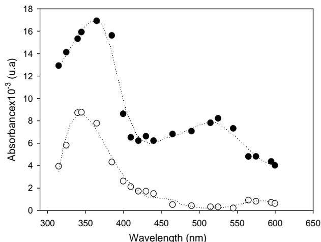
**Fig. 5.** Transient absorption spectra of aqueous deoxygenated solutions of BP (0.1 mM) and NaBr (2 mM) at room temperature recorded after laser excitation ( $\lambda=355$  nm). The filled circles represent the initial spectrum (1  $\mu$ s after the pulse) of (BP+Br<sup>-</sup>) and the empty circles represent the absorption spectrum of the new transient 8  $\mu$ s after the pulse.
