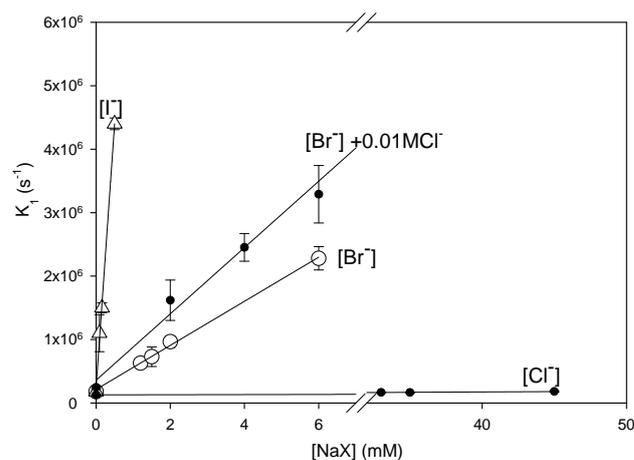
**Fig. 3.** Stern-Volmer plot of the pseudo-first order rate constants as a function of the anion concentrations for the quenching of BP triplet state in deoxygenated aqueous solutions monitored at 525 nm at room temperature. Benzophenone concentration (0.1 mM) laser energy 25 mJ. Error bars are calculated as three times the standard deviation of the least squares slope from analysis.
