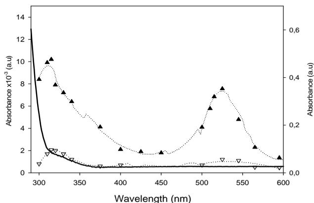
**Fig. 2.** Transient absorption spectra of aqueous deoxygenated solutions of BP (0.1 mM) at room temperature recorded after the 355 nm laser pulses. The filled and empty triangles represent respectively the BP triplet state at 1  $\mu$ s and 8  $\mu$ s after the pulse. The absorption spectrum of the employed benzophenone Aldrich in solution ( $10^{-4}$  M) is shown as a solid line (right scale).
