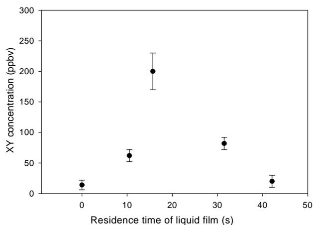
**Fig. 6.** Kinetics of the gaseous dihalogen production as a function of residence time of liquid film in the irradiated flow-tube. The experiments are performed under UV irradiation (spectral irradiance  $1.2 \times 10^{15}$  photons  $\text{cm}^{-2} \text{s}^{-1}$  in the 340–420 nm range) and the conditions were as follow: ambient temperature,  $[\text{BP}] = 100 \mu\text{M}$ ,  $[\text{NaBr}] = 0.01 \text{ M}$ ,  $[\text{NaCl}] = 0.5 \text{ M}$ .
