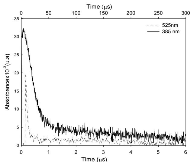
**Fig. 4.** Transient decay at 525 nm (dotted line, bottom scale) and 385 nm (solid line, top scale) obtained after irradiating with 355 nm laser pulse a deoxygenated solution containing 0.1 mM of benzophenone and 0.5 mM of potassium iodide in acetonitrile media.
