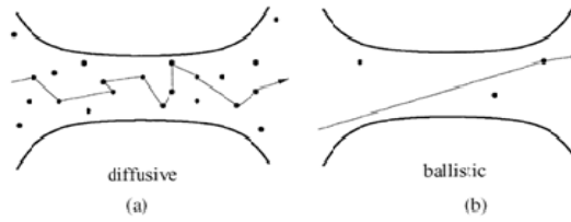
Figure 4: Schematic illustration of (a) diffusive and (b) ballistic electron transport in a conductor [19]
