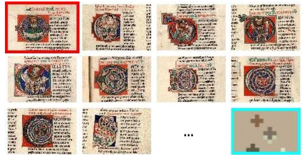
Fig. 12. The query and the first 9 matches (among a total of 90 matches) for the upper point in Figure 11. The spatial organization of colors of the matches is very similar to the one of the query, denoting the presence of a large series of similar images in the database. The last thumbnail (framed in blue) is the background model thumbnail retained to compute the matching threshold.
