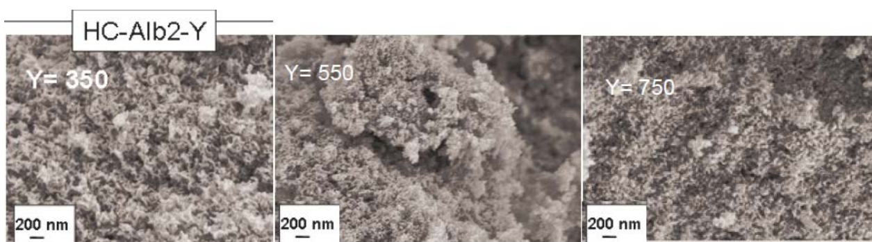
(ESI) Figure 4 – (ESI) Figure 4 – SEM images for further carbonized samples HC-Alb2-Y (Y=350, 550,750). Scale bar is 200 nm.
