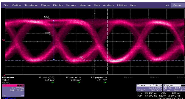
Figure 15. Eye diagram from 875 Mbps demodulated signal (10 m Tx-Rx distance)
