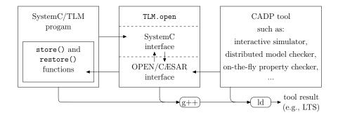
Figure 2: Overview of the verification framework.
