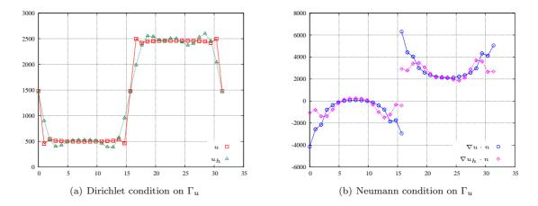
Figure 11: Exact ( $\Box$  resp.  $\bigcirc$ ) and Identified ( $\triangle$  resp.  $\diamond$ ) temperature and flux respectively on  $\Gamma_u$  with noisy data, a = 4%, h = 0.1.
