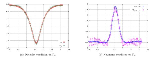
Figure 10: Exact ( $\Box$ ) and identified ( $\odot$ ) boundary conditions with noisy data, r = 1.1, a = 4%, h = 0.02
