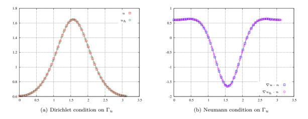
Figure 3: Exact ( $\Box$ ) and identified ( $\odot$ ) boundary conditions, h = 0.03
