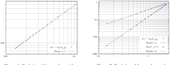
Figure 6: Evolution of  $||u - u_h||_{1,\Omega}$  with respect to h
