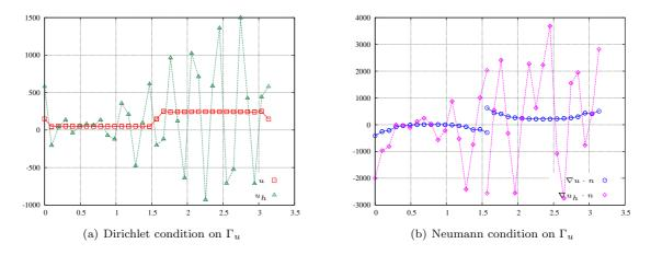
Figure 12: Exact ( $\Box$  resp.  $\bigcirc$ ) and Identified ( $\triangle$  resp.  $\diamond$ ) temperature and flux respectively on  $\Gamma_u$  with noisy data and classical stopping criteria, a = 10%, h = 0.1.
