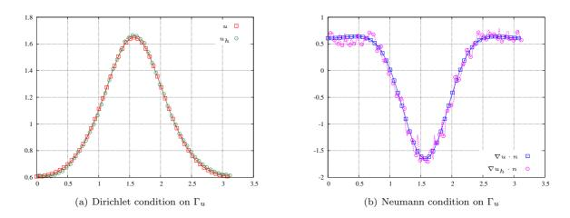
Figure 8: Exact ( $\Box$ ) and identified ( $\odot$ ) boundary conditions with noisy data, a = 4%, h = 0.03
