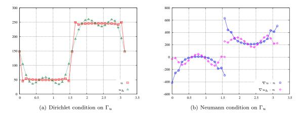
Figure 13: Exact ( $\Box$  resp.  $\bigcirc$ ) and Identified ( $\triangle$  resp.  $\diamond$ ) temperature and flux respectively on  $\Gamma_u$  with noisy data, a = 10%, h = 0.1.
