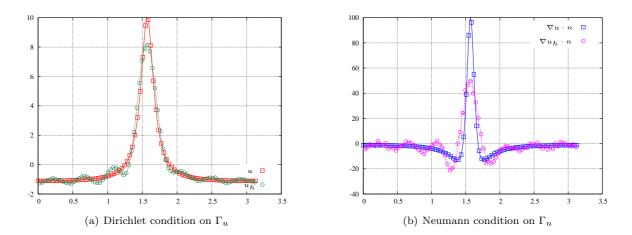
Figure 9: Exact ( $\Box$ ) and identified ( $\odot$ ) boundary conditions with noisy data, r = 0.4, a = 4%, h = 0.02
