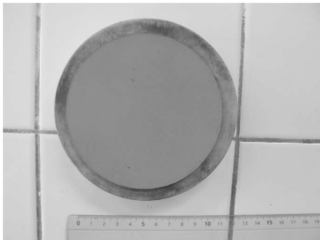
Fig. 10. Photograph of a green iron pellet pressed under 30 MPa, diameter = 120 mm; green porosity = 67%.
