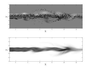
Figure 37: Evaporating polydisperse spray, high inertia droplets, Stokes from 0.48 to 1.1 corresponding to diameters  $d = 60 \ \mu m$  to  $d = 90 \ \mu m$ , at time t=15: (top) Lagrangian particle positions with 7,000 particles over gas vorticity, (bottom) Eulerian number density with a  $400 \times 200 \times 10$  grid.
