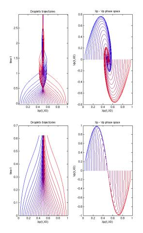
Figure 1: (top) :  $S_t = 0.3$ ,  $S_t > S_{t_c}$ , characteristic crossing in the (x, t) plane (left) and phase plane dynamics (x, v) (right) for 30 initial conditions equally distributed in space with zero initial velocity; (bottom) :  $S_t = 0.03$ ,  $S_t < S_{t_c}$ , no characteristic crossing in the (x, t) plane (left) and phase plane dynamics (x, v) (right) for 30 initial conditions equally distributed in space with zero initial velocity.
