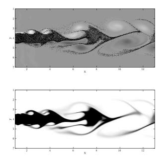
Figure 32: Evaporating polydisperse spray, Stokes 0.011 to 1.1 corresponding to diameters  $d = 9 \,\mu m$  to  $d = 90 \,\mu m$ , at time t=20, : (top) Lagrangian particle positions with 30000 particles, (bottom) Eulerian total number density with a  $400 \times 200 \times 5$  grid.
