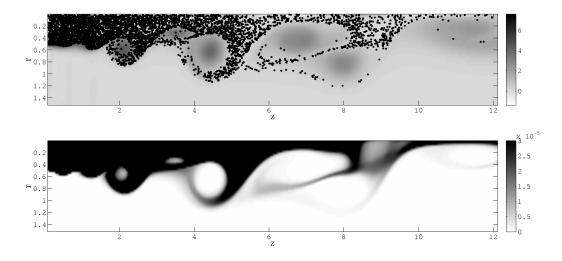
Figure 15: Evaporating polydisperse spray, low inertia droplets, Stokes 0.003 to 0.18 corresponding to diameters  $d = 4 \mu m$  to  $d = 30 \mu m$ , at time t=15: (top) Lagrangian particle positions with 10000 particles, (bottom) Eulerian number density with a  $400 \times 200 \times 5$  grid.
