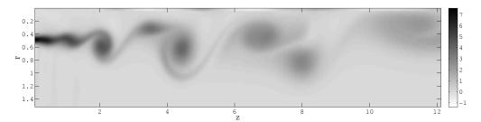
Figure 10: Gaseous vorticity at time t=15, obtained with a low mach number dilatable solver on a  $400 \times 200$  grid.
