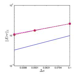
Figure 9: Logarithm of  $L^1$  norm of the error between Eulerian simulation for inertial droplets (ninth section  $S_t = 0.78 S_{t_c}$ ) for various  $\Delta S$  at fixed  $\Delta x$  and the Lagrangian reference solution at time t = 1.5 projected on the comparison grid  $100 \times 100 \times 10$  in the evaporating case : slope one line (blue solid line),  $\Delta x = 1/100$  (magenta solid line),  $\Delta x = 1/200$  (dashed line) and  $\Delta x = 1/400$  (dotted-dashed line).
