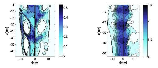
Figure 26: Comparison between experimental measurements - averaged field obtained from 20 instantaneous phase-locked samples (right half) for a 59×44 mm<sup>2</sup> field of view and numerical simulations on a 400 × 400 grid (left half): decane droplet concentration (droplet/mm<sup>3</sup> - left) and mean droplet axial velocities (m.s<sup>-1</sup> - right) for the phase  $\phi = 0$  (arbitrary reference).
