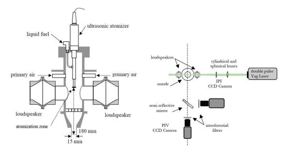
Figure 25: (left) Lateral view of the experimental setup, (right) PIV and IPI experimental set-up.
