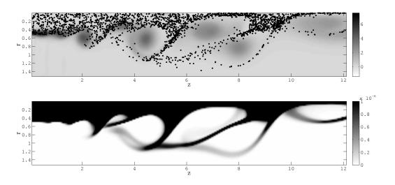
Figure 13: Non-evaporating polydisperse spray, high inertia droplets, Stokes 0.71 to 4.45 corresponding to diameters  $d = 60 \,\mu m$  to  $d = 150 \,\mu m$ , at time t=15: (top) Lagrangian particle positions with 40000 particles, (bottom) Eulerian total number density with a  $400 \times 200 \times 5$  grid.
