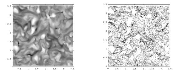
Figure 42: Eulerian-Lagrangian comparisons in the plane (x - y) at z = 1.75 for low inertia droplets, St = 0.17: (left) Eulerian multi-fluid number density, (left) Lagrangian droplet positions.
