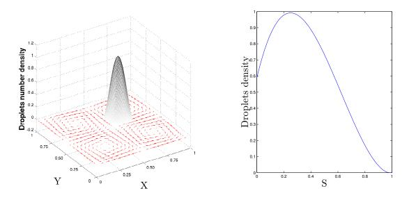
Figure 3: Initial droplet distribution : (left) non uniform spatial repartition, three-dimensional plot with number density as the third coordinate; (right) non-dimensional polydisperse size distribution.
