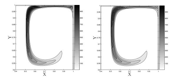
Figure 4: Zoom on the top-right quarter of the periodic computational domain of the total mass density of droplets at time t = 1.5, projected on the comparison grid  $100 \times 100 \times 10$ : (left) Lagrangian reference solution, (right) Eulerian with a  $400 \times 400 \times 10$  grid.
