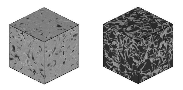
Figure 38: Eulerian spray number density at the edges of the domain, obtained with the multi-fluid method on a  $129^3$  Cartesian grid : (left) St = 0.17, (right) St = 1.05.
