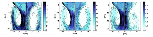
Figure 27: Comparison between IPI experimental measurements - averaged field obtained from 120 instantaneous phase-locked samples with a reduced field of view of  $27 \times 20 \text{ mm}^2$  (right half) and numerical simulations on a 400 × 400 grid (left half): total droplet concentration at phase  $\pi$  in droplet/mm<sup>3</sup>; from left to right: decane (non evaporating reference liquid), methanol and heptane (evaporating liquids).
