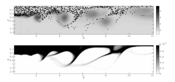
Figure 16: Evaporating polydisperse spray, high inertia droplets, Stokes 0.71 to 4.45 corresponding to diameters  $d = 60 \,\mu m$  to  $d = 150 \,\mu m$ , at time t=15: (top) Lagrangian particle positions with 10000 particles, (bottom) Eulerian total number density with a  $400 \times 200 \times 5$  grid.
