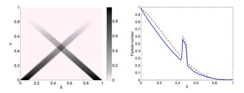
Figure 24: Total droplet number density of evaporating jets crossing simulated with high order moment methods for size and velocity at t = 1 on a  $100 \times 100$  grid (left) and comparison of the number density of the numerical solution (solid line) and the analytical solution (dashed line).
