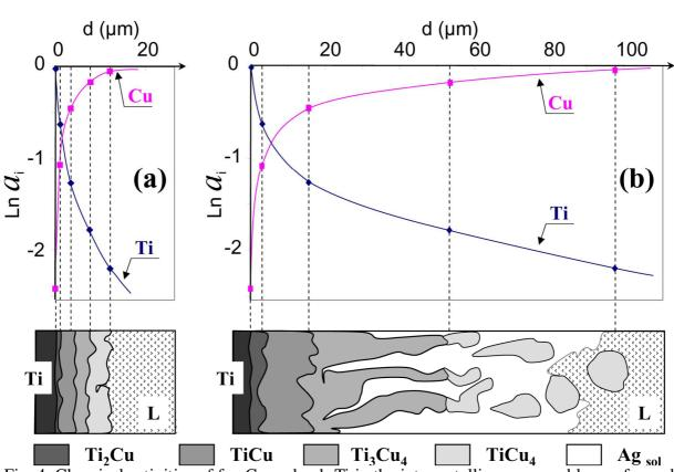
Fig. 4. Chemical activities of fcc-Cu and cph-Ti in the intermetallic compound layers formed by reaction at 790 °C of solid titanium with (a) pure and (b) Ti-saturated Ag-40 at.% Cu liquid alloy
