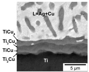
Fig. 2. Thin reaction zone formed between solid Ti and titanium-free Ag-40 at.% Cu liquid alloy after 50 min of heating at 790  $^{\circ}\text{C}$
