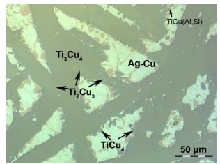
Fig. 5.  $Ti_3Cu_4$  plate-like crystals grown in mixture F first reacted at 825 °C for 353 h and then annealed at 854 °C for 50 min (note the difference with Fig. 3)
