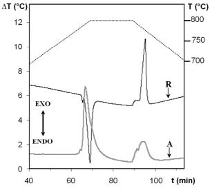
Fig. 8. Thermal behaviour upon first cycle of two cold-pressed powder mixtures analysed by SDTA at 4 °C.min<sup>-1</sup>: mixture R with composition Ag:Cu = 60:40 at% and mixture A with composition Ag:Cu:Ti = 43:28.5:28.5 at% (temperature versus time is drawn in the upper part of the graph)
