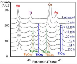
Fig. 6. Evolution of the XRD pattern of mixture F placed for increasing times in a tubular furnace held at the constant temperature of 790  $^{\circ}$ C
