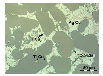
Fig. 3.  $Ti_2Cu_3$  globular crystals in a silver-rich matrix, as synthesized in mixture F after heating at 825 °C for 353 h: small crystals in the matrix analyse for TiCu(Al,Si) whereas TiCu<sub>4</sub> crystals are stuck onto Ti<sub>2</sub>Cu<sub>3</sub>
