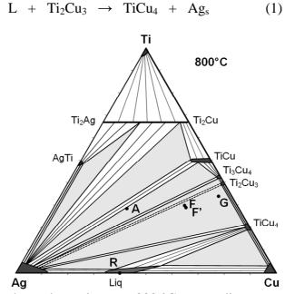
Fig. 1. Ag-Cu-Ti isothermal section at 800 °C, according to experimental data and thermodynamic evaluations [6-16]. The tie lines joining Ag<sub>s</sub> to  $Ti_2Cu_3$  have been drawn in dotted lines since for Eremenko et al. [6-8],  $Ti_2Cu_3$  is not stable at 800 °C
