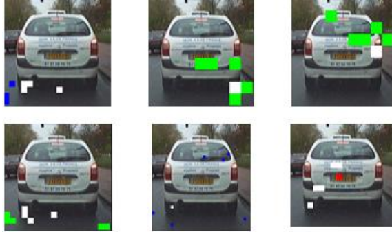
AdaBoost trained Control-Points features for vehicle detection .This result was obtained from 500 positive and 1000 negative examples set training.
