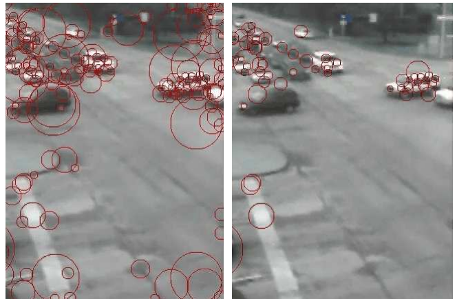
Fig. 13. First detection test on a video: all keypoints on the left side, and only positively-reponding keypoints on the right side.
