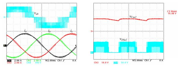
Fig. 6: Experimental results for  $v_{ab}$ ,  $i_a$ ,  $i_b$ ,  $i_c$ ,  $v_{Csa2}$ , and  $v_{DSa2}$  in the following conditions:  $V_{dc} = 150 \text{ V}$ , m = 0.95,  $C = 155 \mu\text{F}$ ,  $C_{sx1} = C_{sx4} = 330 \text{ nF}$ ,  $C_{sx2} = C_{sx3} = 330 \text{ nF} + 10 \mu\text{F}$  ( $x \in \{a, b, c\}$ ), switching or carrier frequency  $f_s = 5 \text{ kHz}$ , and a linear and balanced load with per-phase impedance  $Z_L = 22.5 \Omega \angle 12^\circ$  (series R-L load).
