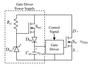
Fig. 3: Gate-driver power-supply circuit ( $x \in \{a, b, c\}$ ,  $i \in \{1, 2, ..., 2n-2\}$ ).
