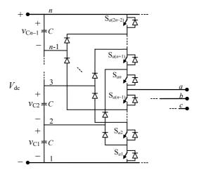
Fig. 1: *n*-level diode-clamped topology with multiple legs.
