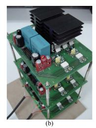
Fig. 5: Three-level three-leg dc-ac converter. (a) Topology. (b) Prototype using 150 V MOSFETs as devices  $S_{vi}$ .
