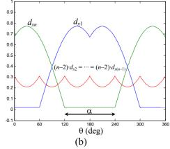
Fig. 4: Leg x duty-ratio pattern for an *n*-level three-leg converter (m = 0.75). (a) Original PWM scheme. (b) Modified PWM scheme with  $d_{\text{offset}} = 0.02$ .
