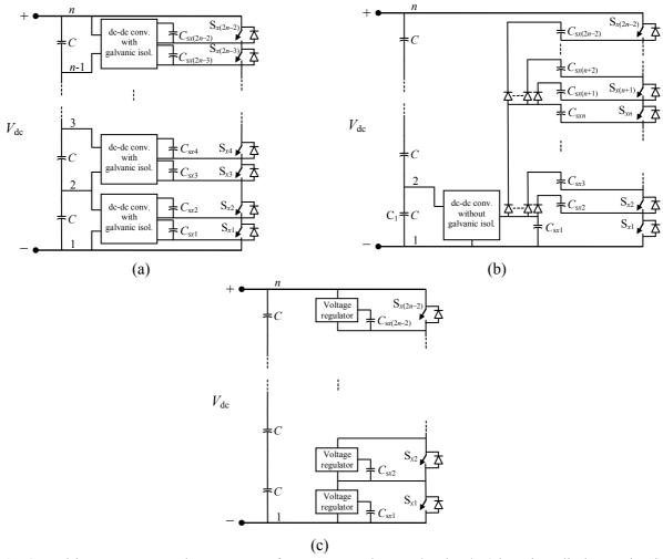
Fig. 2: Gate-driver power-supply structures for converter leg  $x \in \{a, b, c\}$  (clamping diodes omitted). (a) Structure 1 based on dc-dc converters with galvanic isolation. (b) Structure 2 based on the bootstrap technique. (c) Structure 3 using voltage regulators connected across the active devices.
