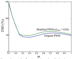
Fig. 12: *THD* in the line-to-line voltage of a five-level three-leg diode-clamped converter as a function of the modulation index m. Conditions:  $f_s / f_o = 100$  and harmonics considered up to  $40 \cdot f_s$ .
