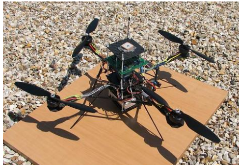
Fig. 1. Our home-built quadrotor: the “Quadricopter”.
