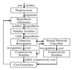
Figure 1. Flow chart of the understanding system.
