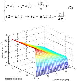
Figure 3. Front lateral force as a function of the sideslip angle and the camber angle.
