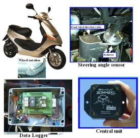
Figure 12. Motorcycle equipment using for validation.
