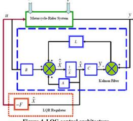
Figure 4. LQG control architecture.
