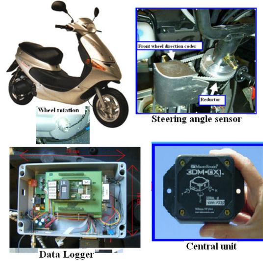
Figure 12. Motorcycle equipment using for validation.
