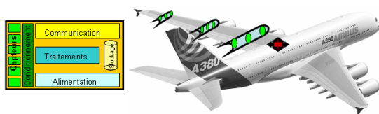
Fig. 1. Structure health monitoring network.
