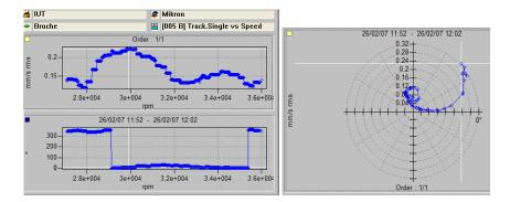
Fig. 4 Tracking signal using speed domain 36000-28000 rpm; direction X-X
