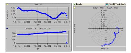
Fig. 5 Tracking signal using speed domain 28000-18000 rpm; direction X-X
