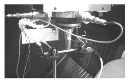
Fig. 3 Accelerometers placement on the spindle of milling machine tool
