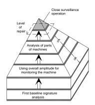
Fig. 2 Elements of typical predictive monitoring program.
