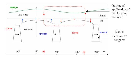
Fig. 1: Developed scheme for a poles pair and the chosen Ampere's theorem path.
