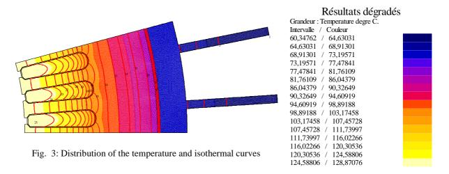
From these isothermal curves we can observe that the stream of heat follows a radial direction. Then, we modeled a network of the thermal resistances under Pspice software. In this model, copper and iron losses are considered as current sources, while temperature in each point is considered as an electrical potential, and thermal resistances are equivalent to the electrical resistances.
