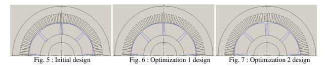
Figs. 5, 6 and 7 are graphical representations of various optimizations; optimization 1 is achieved with a fixed bore diameter and optimization 2 with a free bore diameter.
