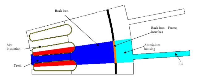
Fig. 2: Geometry used to establish the thermal model
