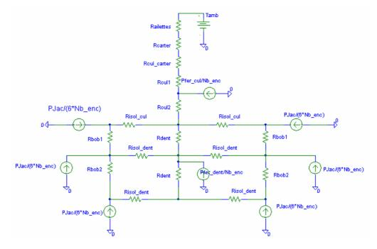
Fig. 4: Network of the thermal resistances
