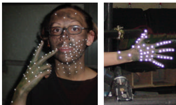
Figure 3. Our female FMCS user and the reflective markers used for the dynamic corpus. She wears 50 markers on her right hand and 63 markers on her face, mainly on her left side.
