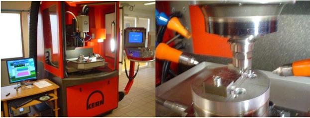
Fig. 3. Experimental data acquisition system used in milling
