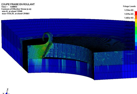
Fig. 2. Von Mises stress contours obtained through simulation results of a milling process numerical model with LS-Dyna software. The cutting conditions are  $N=20000\text{rpm}$ ;  $f_t=0,3\text{mm/tooth}$ ;  $V_c=250\text{m/min}$ .
