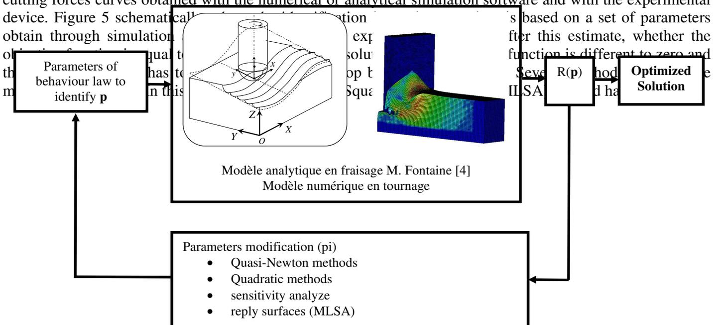
Fig. 5. Diagram representing the inverse identification procedures.
