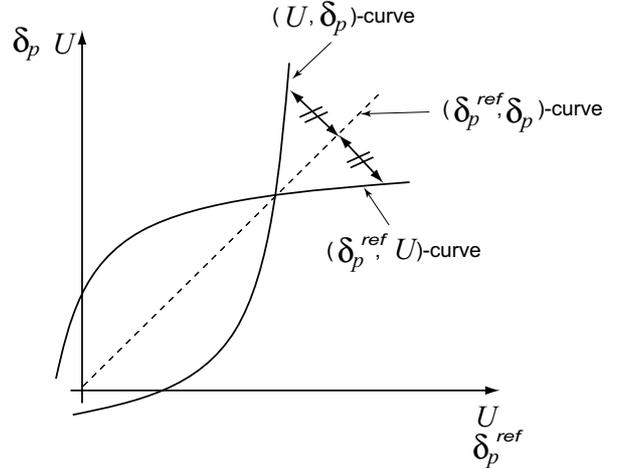
Fig. 7. Schemes showing the compensation of a hysteresis [11].
