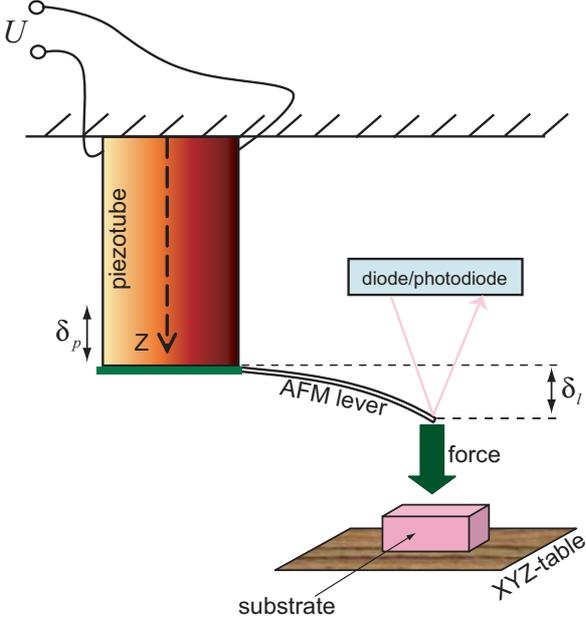
Fig. 2. Principle of the force measurement system.
