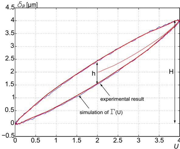
Fig. 8. Hysteresis curves: experimental result and identification result.
