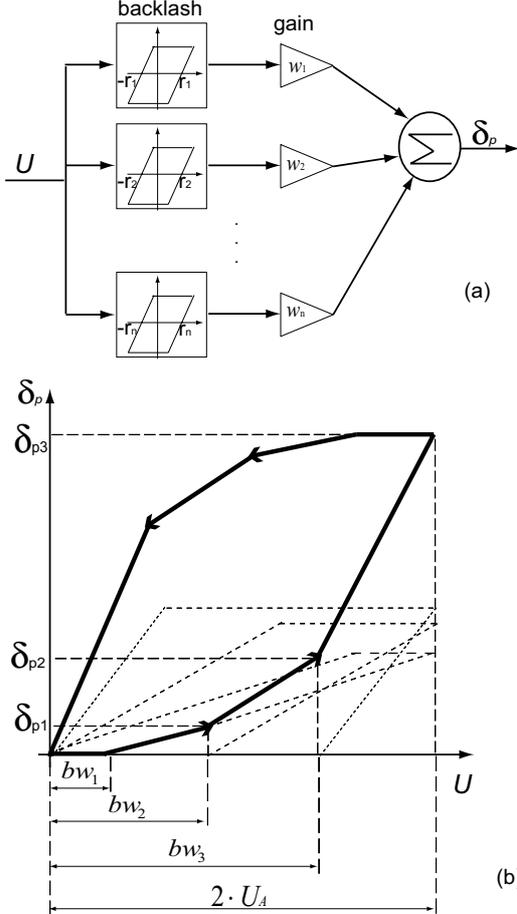
Fig. 6. Schemes showing the principle of the PI model.
