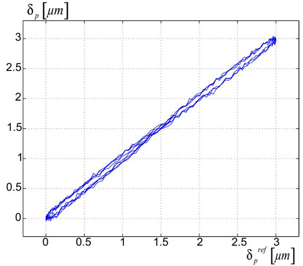
Fig. 9. Experimental result of the hysteresis compensation.
