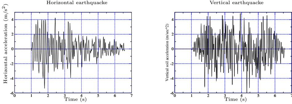
Fig. 6. Horizontal (left) and vertical (right) earthquake components applied on the foundation.
