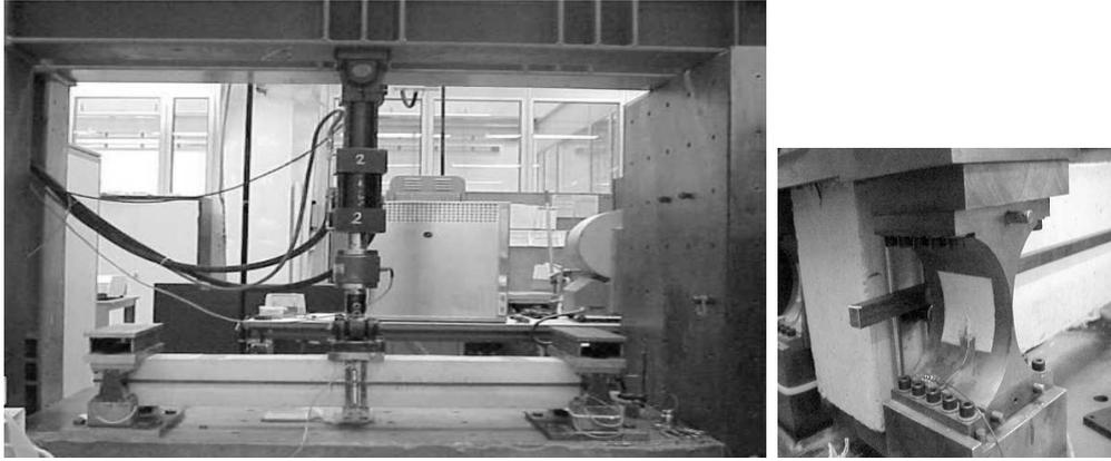
Fig. 7. Experimental setup (left) and hinge device (right).
