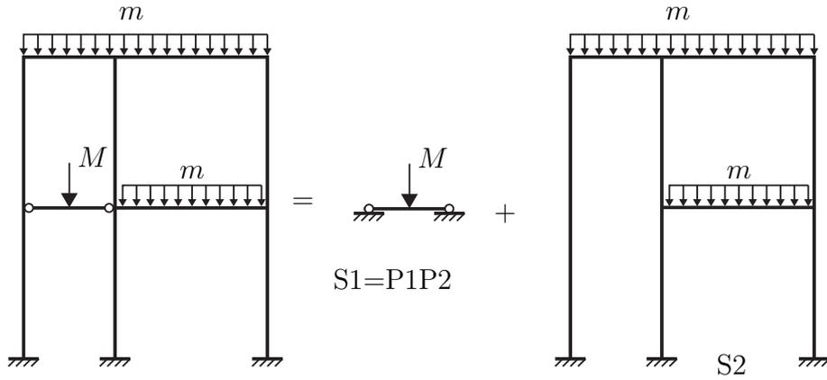
Fig. 5. Decomposition of the structure into tested substructure S1 and simulated substructure S2.
