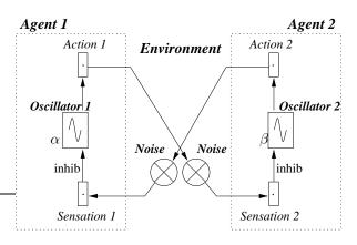
Fig. 2. Architecture of the two agents influencing each other. Each agent is driven by an internal oscillator and produces actions depending on this oscillator. A noise due to the environment and the hardware devices appears on the signal between the two oscillators.
