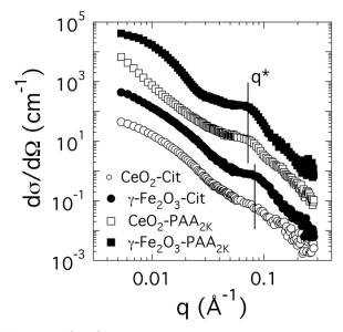
**Figure 2**: SANS cross-sections of nanoparticle-copolymer clusters comparing citrate and PAA<sub>2K</sub>-coated CeO<sub>2</sub> and γ-Fe<sub>2</sub>O<sub>3</sub>. The total concentrations were c = 5.8, 2, 11 and 1.7 wt. % for the clusters made with CeO<sub>2</sub>-Cit, γ-Fe<sub>2</sub>O<sub>3</sub>-Cit, CeO<sub>2</sub>-PAA<sub>2K</sub> and for γ-Fe<sub>2</sub>O<sub>3</sub>-PAA<sub>2K</sub> respectively. The intensities were shifted upwards by coefficients 1, 3, 2 and 500.
