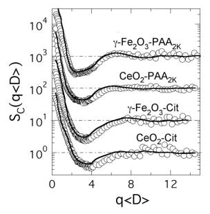
**Figure 4**: Internal structure factors of clusters as a function of the product  $q\langle D\rangle$ , where  $\langle D\rangle$  is the average nanoparticle diameter. Continuous lines are from Reverse Monte Carlo simulations. There, the single particles were described as polydisperse and obeying the size distributions found experimentally.
