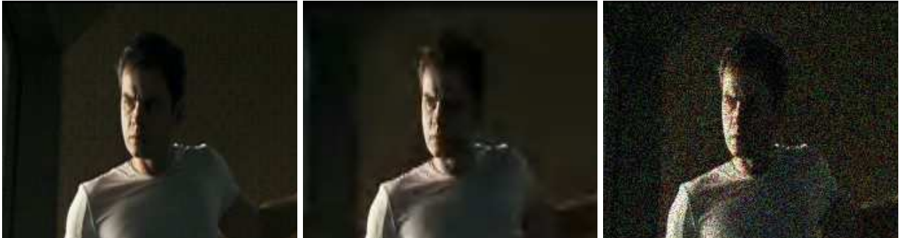
Figure 12: Detail of frame 1 of sequence “Poltergay” ( in lexicographical order ) uncorrupted, corrupted by JPEG2000 compression artifacts, and corrupted by a Gaussian noise.
