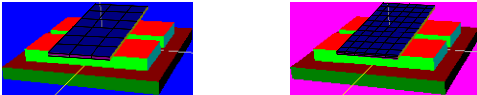
Fig. 8 – discretizing for coarse model is 6 \times 3 \times 1 = 18 blocks, for fine model 12 \times 6 \times 2 = 144 blocks
