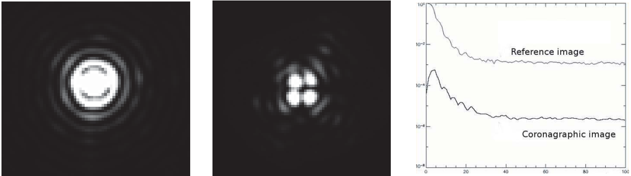
Fig. 3. Reference image ( left ), Coronagraphic image \times 1000 ( center ) and overage radial profiles ( right ).
