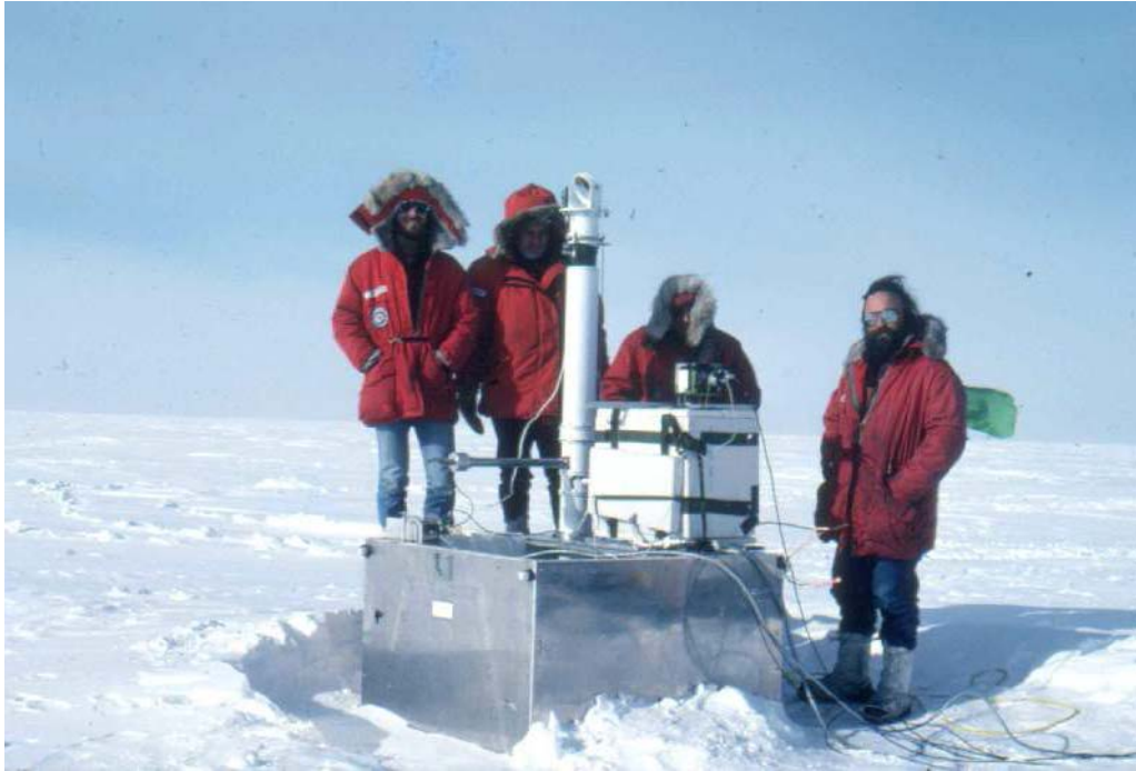
Fig. 1. From left to right, Eric Fossat, Martin Pomerantz, Lyman Page and Gerard Grec with the first solar both azimuthal and equatorial telescope that was successfully operated at the geographical South Pole in 1979/1980, providing 6 days of uninterrupted full disk oscillation data
