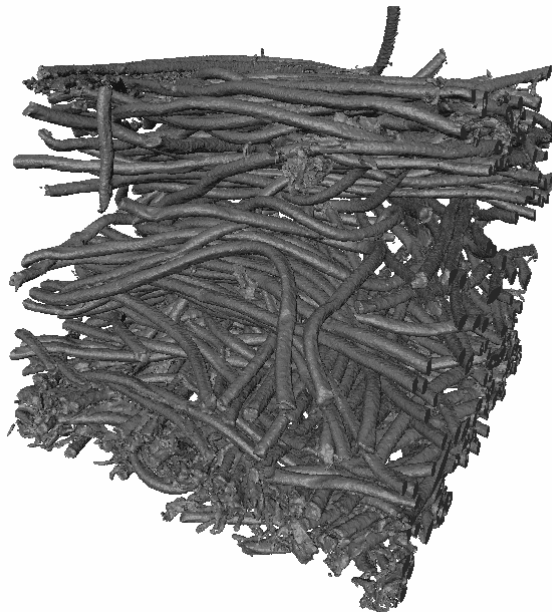
Figure 5 Example of image of GDL microstructure obtained by X ray microtomography
