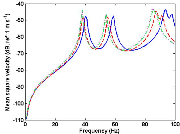
**Figure 3.** Convergence of FEM in heavy fluid - Comparison of mean square velocity obtained by direct resolution for 4 mesh criteria: (-)  $\frac{\lambda}{6}$ , (- -)  $\frac{\lambda}{12}$ , (-.-)  $\frac{\lambda}{28}$  and (...)  $\frac{\lambda}{60}$
