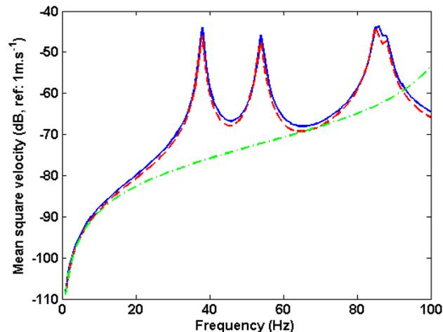
**Figure 4.** Residual shapes effect - Comparison of mean square velocity for: (-) FEM solution ( $\frac{\lambda}{28}$ ), (-.-) PTF method without residual shapes ( $\frac{\lambda}{6}$ ) and (- -) PTF method introducing residual shapes ( $\frac{\lambda}{6}$ )
