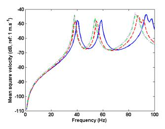
**Figure 3.** Convergence of FEM in heavy fluid - Comparison of mean square velocity obtained by direct resolution for 4 mesh criteria: (-)  $\frac{\lambda}{6}$ , (- -)  $\frac{\lambda}{12}$ , (-.-)  $\frac{\lambda}{28}$  and (...)  $\frac{\lambda}{60}$
