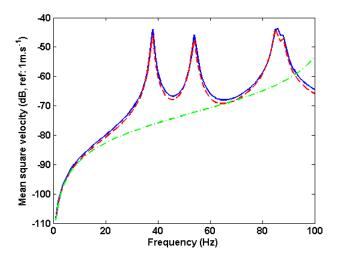
**Figure 4.** Residual shapes effect - Comparison of mean square velocity for: (-) FEM solution  $(\frac{\lambda}{28})$ , (-.-) PTF method without residual shapes  $(\frac{\lambda}{6})$  and (- -) PTF method introducing residual shapes  $(\frac{\lambda}{6})$
