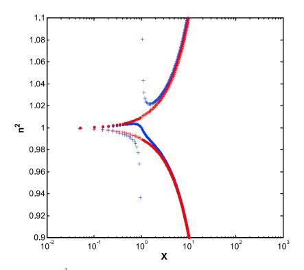
**Figure 8.** Dependence of  $n^2$  on X for a cold collisionless electron plasma when Y = 100. Red curves are for  $\theta = 0^\circ$ , and blue curves are for  $\theta = 10^\circ$ . The  $n^2$  solutions are derived from the Appleton-Lassen formula. Pluses and dots refer to the positive and negative signs in the denominator of the second term, respectively.
