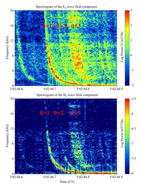
**Figure 4.** DEMETER VLF measurements on 28 July 2005 around 0502:44 UT. The most intense 0+ whistlers simultaneously observed on the spectrogram of (top)  $E_x$  electric field component and (bottom)  $B_y$  magnetic field component are at 0502:44.685 UT and 0502:44.723 UT and start at 0502:44.753 UT for a cluster of 0+ whistlers. There is an uncertainty on the DEMETER UT time of the order of 10 ms.
