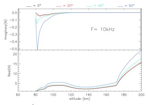
**Figure 9.** Variation of  $n^2$  with altitude *h* for f = 10 kHz. The electron plasma frequency profile is that of Figure 7. The electron collision frequency profile is given by  $v = 1.816 \times 10^{11} \exp \{-0.15h\}$ . Calculations are made for  $\theta = 0^{\circ}$ ,  $20^{\circ}$ ,  $40^{\circ}$ , and  $60^{\circ}$ .
