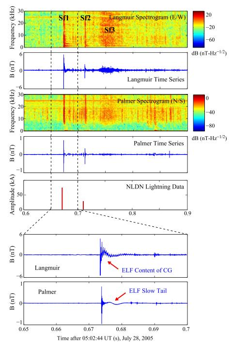
**Figure 3.** VLF/ELF ground-based measurements on 28 July 2005 around 0502:44 UT. Sferic 1 is observed at 0502:44.671 UT, sferic 2 at 0502:44.709 UT, and sferic 3 is in fact a cluster of sferics starting around 0502:44.740 UT.
