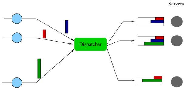
Figure 1: Centralized architecture for a server farm.
