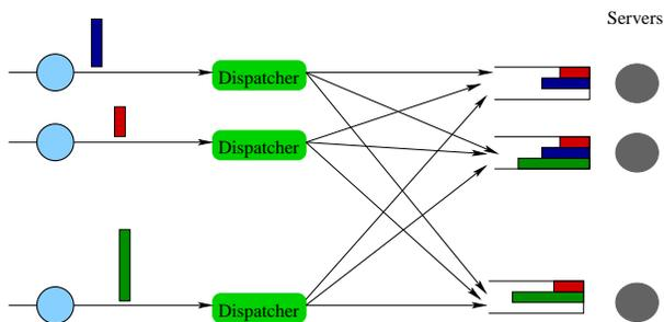
Figure 2: Decentralized architecture for a server farm.
