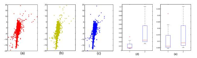
Fig. 2 DINOSAUR DATA: (a)-(c) Upper view of the 3D points estimated by the KK-procedure (a), by the SH-procedure (b) and by our procedure. (d) Boxplots of the errors when estimating the camera centers by our procedure (left) and by the KK-procedure (right). (e) Boxplots of the errors when estimating the camera centers by our procedure (left) and by the SH-procedure (right).
