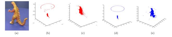
Fig. 1 (a) One image from the dinosaur sequence. (b)-(c) Camera locations and scene points estimated by the blind  $L_{\infty}$ -cost minimization. (d)-(e) Camera locations and scene points estimated by the proposed "outlier aware" procedure. This figure demonstrates that the estimator minimizing the  $L_{\infty}$ -cost is severely affected by the outliers.
