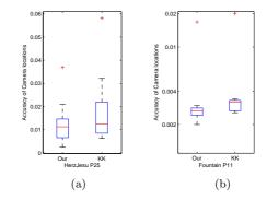
Fig. 5 Boxplots of the errors when estimating the camera centers by our procedure (left) and by the KK-procedure (right) for (a) HerzJesu P25 sequence and (b) Fountain P11 sequence.
