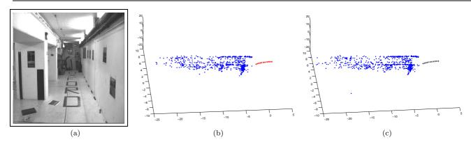
Fig. 3 CORRIDOR DATA: (a) One image out of 11. (b) Camera locations and scene points estimated by our method. (c) True cameras and scene points.
